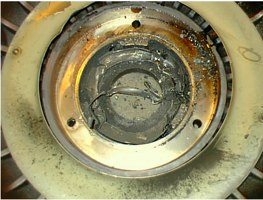
Motor removed due to DE bearing failure 3/17/2003
