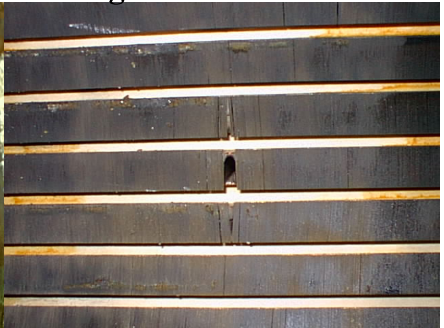
Motor removed due to DE bearing failure 3/17/2003
