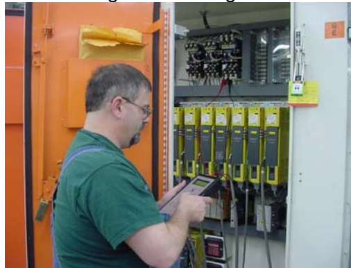
Figure 7: Testing A Machining Center with MCA
