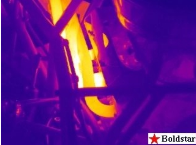
Image: Infrared image of late model stock car performance engine exhaust
